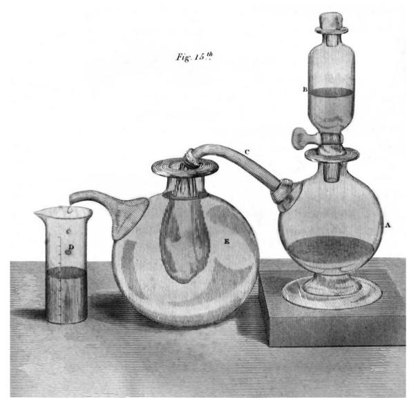
**FIGURE 283.** • Humphry Davy's apparatus for measuring the amount of limestone in soil. Sulfuric acid releases one equivalent of  $CO_2$  from an equivalent of limestone (CaCO<sub>3</sub>). The gas fills a balloon, displacing a volume of water that is measured to give the volume of gas generated. (From Davy, *Agricultural Chemistry*, London, 1813.)
