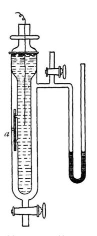
**FIGURE 280.** Schematic of the apparatus used by J.L. Soret in 1872 to elucidate the formula  $(O_3)$  of ozone—see text for explanation (from Partington, *Everyday Chemistry*, 1929, MacMillan and Co., Ltd, London). It is quite amazing that the formula of this highly energetic, highly reactive trace component of the atmosphere was solved more than 130 years ago.
