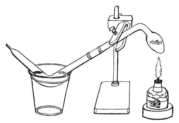
**FIGURE 244.** Ede's very simple and elegant student experiment for obtaining and trapping at 0°C, the deep blue, highly unstable dinitrogen trioxide ( $N_2O_3$ ), which decomposes at only 3°C. This would still be a nice experiment today, almost 170 years later. (See Figure 243.)
