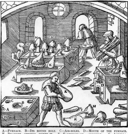
A-FURNACE. B-ITS ROUND HOLE. C-AIR-HOLES. D-MOUTH OF THE FURNACE. E-DRAUGHT OPENING UNDER IT. F-EARTHENWARE CRUCIBLE. G-AMPULLA. H-OPERCULUM. I-ITS SPOUT. K-OTHER AMPULLA. L-BASKET IN WHICH THIS IS USUALLY PLACED LEST IT SHOULD BE BROKEN
