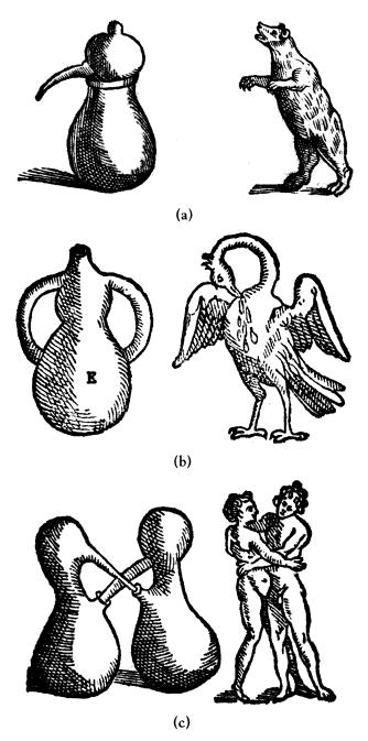
**FIGURE 72.** Depictions of glassware and metaphors from Porta's *De Distillatione* (Figure 70): (a) Distillation apparatus employing a distillation head (alembic) atop a wide-mouth flask (or cucurbit) along with matching bear; (b) one-piece pelican for refluxing a liquid and the pelican itself biting its chest—considered a blood of Christ symbol; (c) A double pelican for prolonged exchange of hot fluids and an interesting metaphor.
