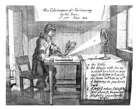
**FIGURE 121.** ■ Calcination of antimony using "celestial fire" (from Le Fèvre's 1670, A *Compleat Body of Chymistry*). Le Fèvre was among the earliest chemists to discover that the calx was heavier than the corresponding pure metal.
