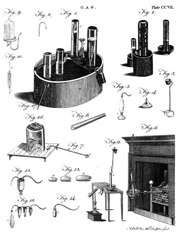
**FIGURE 198.** ■ Collage of Joseph Priestley's pneumatic apparatus. A gun barrel is used as reaction chamber and placed in a fireplace. The resulting gases, if water-soluble, are collected over mercury (*Fig. 11*).
