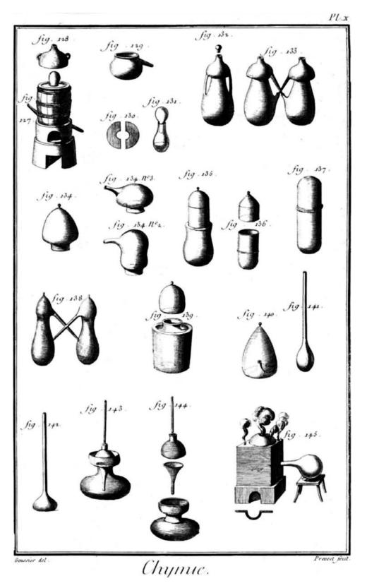
**FIGURE 191.** ■ Various types of recirculation apparatus (see text) from the eighteenthcentury encyclopedia published by Diderot and D'Alembert.
