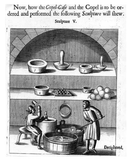
**FIGURE 26.** Manufacture of cupels (using a paste made from crushed bone and beer) from Pettus' 1683 *Fleta Minor*. Compare this figure with the corresponding one (Figure 9) in the 1736 edition (i.e., the original 1574 edition), and you will note that costumes have been updated by a century while the apparatus remains unchanged.
