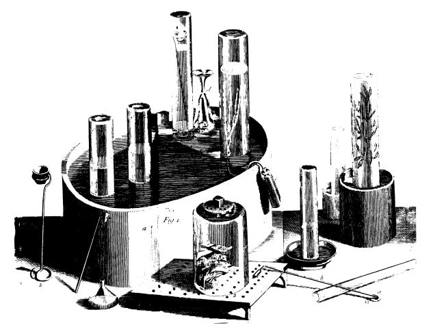
**FIGURE 197.** ■ Joseph Priestley's pneumatic trough for isolation of "factitious airs" (gases derived from solids). Although Scheele was the first to discover oxygen, Priestley published first (1774). He was gentle to his experimental mice (from the later abridged edition, *Experiments and Observations on Different Kinds of Air*, Birmingham, 1790).
