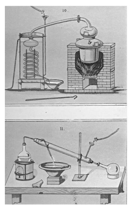
**FIGURE 253.** Black and white image of a color plate from the 1854 American edition of *Notions Générale de Chimie* by Pelouze and Fremy. See color plates. Depicted in *10* is an industrial-scale still consisting of a copper boiler covered with a hood; *11* displays the very modern-looking water-cooled distillation apparatus designed by Gay-Lussac.
