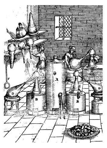
**FIGURE 13.**  $\blacksquare$  The use of "parting acid" (mostly HNO<sub>3</sub>) to separate silver from gold. Silver is soluble and gold is not soluble in this acid (Ercker, see Figure 5).
