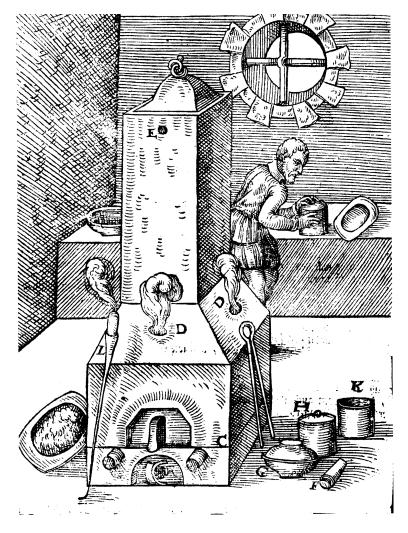
**FIGURE 14.** ■ A sixteenth-century self-stoking cementation furnace (see text; Ercker, see Figure 5).
