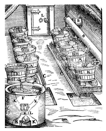
**FIGURE 16.** ■ Steps in the leaching and concentration (by boiling) of saltpetre obtained from old sheep dung (Ercker, see Figure 5).
