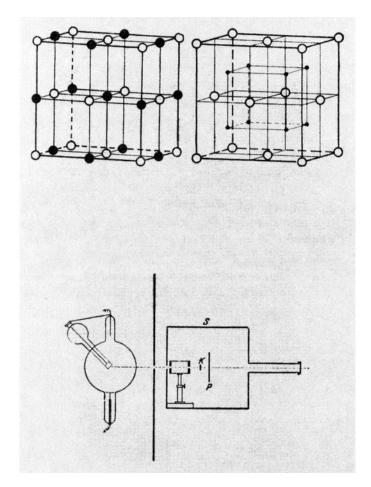
**FIGURE 309.** ■ Shortly after x-rays were discovered by Röntgen, Max von Laue postulated that their wavelengths were similar to the separations between atoms in ionic crystals such as rock salt and fluorspar (top). His x-ray unit is pictured at bottom (from Max Born, *The Constitution of Matter* (London, 1923).
