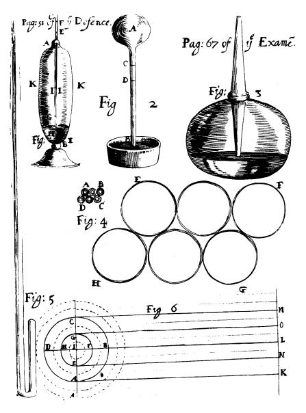
**FIGURE 146.** In *Fig. 5* we see Robert Boyle's famous J tube used to demonstrate that PV = k (Boyle's Law). Air is trapped by mercury in the small arm of the J tube. As more mercury is added, the volume of the air decreases. (From *New Experiments Physico-Mechanical* . . . , 1662).
