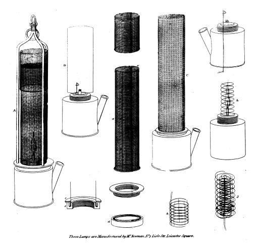
**FIGURE 246.** ■ Depictions of aspects of Humphry Davy's Safety Lamp for Coal Miners (London, 1818). His ingenious solution to lamps that would ignite coal gas with deadly results was incredibly simple. The fine metallic mesh would cool the coal gas below its flash point. Thus, although the flame and combustible gas were in open contact, there would be no explosion.
