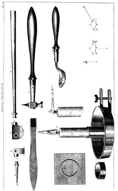
**FIGURE 171.** Apparatus employed in blowpipe analysis of minerals was developed to a high state of technology in eighteenth-century Sweden (from Torbern Bergman's 1788 *Physical and Chemical Essays*).
