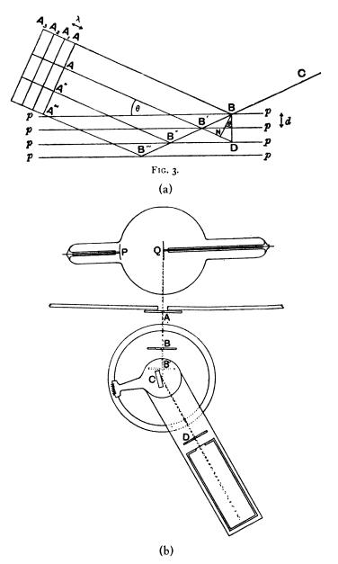
**FIGURE 316.** ■ William H. Bragg and his son William L. Bragg reversed von Laue's experiment and used x-rays to measure the distances between ions or atoms in crystals (see text), (a) Depicts the conditions for constructive interference of x-rays termed *Braggs' Law;* (b) schematic of Braggs's x-ray apparatus (W.H. Bragg and W.L. Bragg, X-Rays And Crystal Structure, 4th ed., London, 1924).
