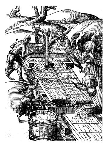
**FIGURE 8.** • A sixteenth-century machine washing alluvial gold ores (Ercker, see Figure 5). Gold's great density (19.3 g/cm<sup>3</sup> permits its ready separation from other, lighter minerals.
