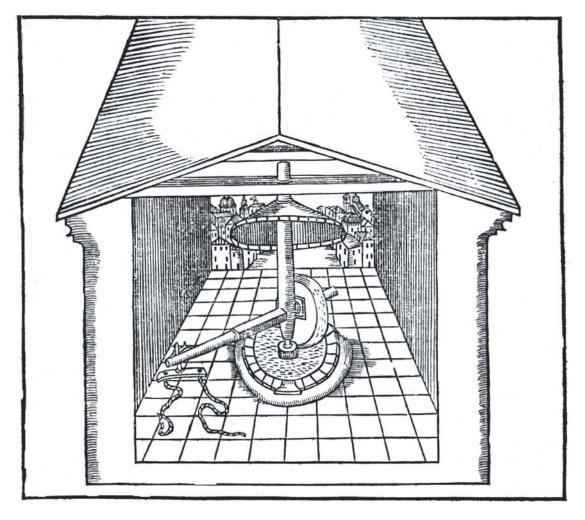
**FIGURE 32.** ■ Mill for grinding the components of gunpowder (ca. 75% saltpetre; the remainder roughly equal parts of charcoal and sulfur) depicted in Bianco's 1598 work on artillery and fireworks (from The Roy G. Neville Historical Chemical Library, a collection in the Othmer Library, CHF).
