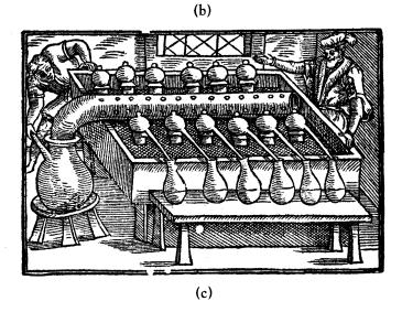
**FIGURE 110.** Distillation apparatus from Gesner's treatise of 1599: (a), left: A furnace employing a water bath is termed the *Bain Marie* (*Balneum Marie* or bath of Marie); (b) heating samples in closed cucurbits using sand heated by the sun preferably in July or August; (c) A heating bath of boar dung freshly steamed. I suggest calling this the "Bane of Marie" and further advise outdoor use only.
