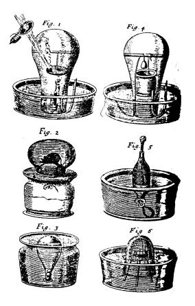
**FIGURE 150.** ■ This plate is from John Mayow's *Tractus Quinque Medico Physici* (Oxford, 1674). It shows his experiments in which "nitro-aerial spirit" in saltpetre was transferred to antimony under a heating glass. In effect oxygen was transferred between the two substances (from the Dr. Roy G. Neville Historical Chemical Library, a collection in the Othmer Library, CHF).
