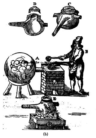
**FIGURE 113.** ■ From French's *The Art of Distillation:* (a), left, glass crystals heated by the sun as heat source; right, iron or marble mortar as the heat source; (b) heavy-duty furnace for distillation from large quantities of bones, horns, minerals, and vegetables.
