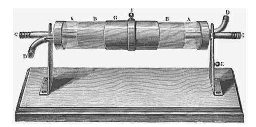
**FIGURE 279.** Illustration of a late-nineteenth-century ozone generator. The apparatus was designed to expose flowing oxygen gas to a "silent discharge" of electricity since sparks decompose ozone (1 mol  $O_3$ ) back to oxygen (1.5 mol  $O_2$ ). (From Roscoe and Schorlemmer, A *Treatise on Chemistry*, 1894.)
