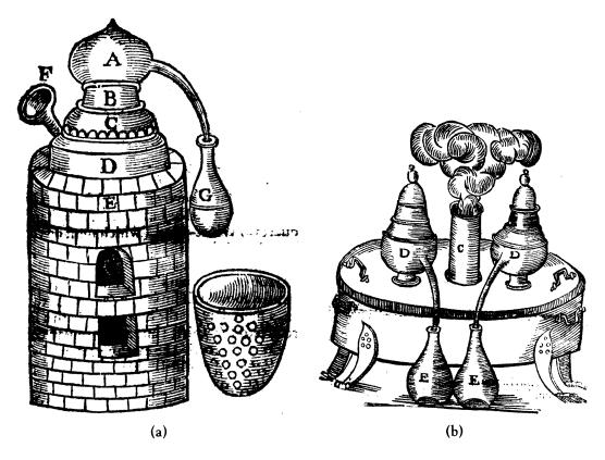
**FIGURE 112.** ■ Apparatus from *The Art of Distillation* by John French (London, 1653; first edition, 1651): (a) Apparatus for steam distillation; (b) A *Balneum Marie*.
