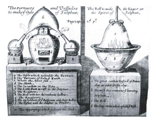
**FIGURE 120.** ■ Distillation of oil of vitriol (sulfuric acid) in tin-lined vessels (from Le Fèvre's 1670 edition, A *Compleat Body of Chymistry*).
