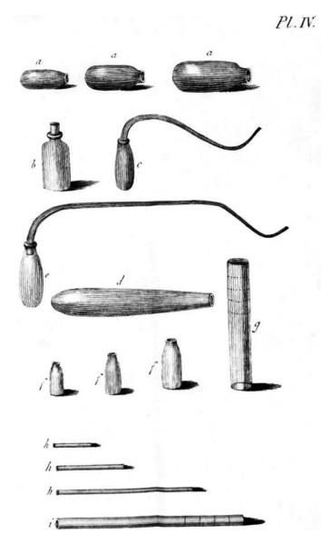
**FIGURE 199.** ■ Drawing g depicts the simplest possible eudiometer (a graduated tube sealed at one end). Measured volumes of gas are introduced and changes in final volume measured. Priestley's earliest eudiometers simply measured the "goodness" (oxygen content) of air by reaction with freshly generated "nitrous air" (actually nitric oxide, NO). (From Priestley, *Experiments and Observations on Different Kinds of Air*, 1790 edition.)
