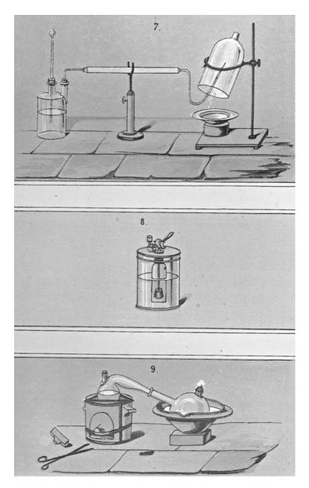
**FIGURE 252.** ■ Black and white image of a color plate from the 1854 American edition of *Notions Générale de Chimie* by Pelouze and Fremy. See color plates. Depicted in 7 is a synthesis of water involving generation of hydrogen and its combustion in air; 8 shows a clever self-controlling hydrogen gas generator; 9 illustrates a laboratory-scale distillation apparatus appropriate for students.
