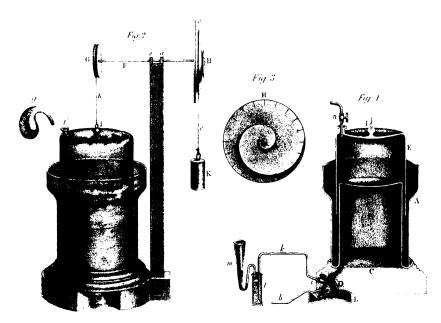
**FIGURE 223.** Diagram of Humphry Davy's apparatus for storing and breathing nitrous oxide (from *Researches*, *Chemical and Philosophical*, *chiefly concerning Nitrous Oxide*, *or Dephlogisticated Nitrous Air, and its Respiration*; the original edition, published in 1800, is of very great rarity). Davy's artistic circle of friends included poet Samuel Taylor Coleridge and Dr. Mark Roget (*Thesaurus* fame) who sampled laughing gas with Davy and recorded their scientific observations.
