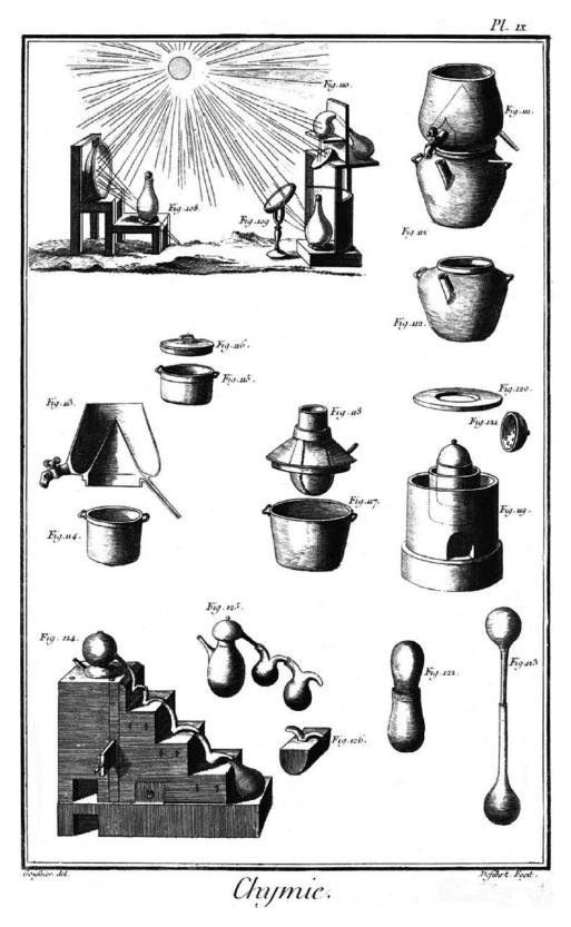
**FIGURE 190.** ■ Distillation and recirculation apparatus (see text) from the eighteenthcentury encyclopedia published by Diderot and D'Alembert.
