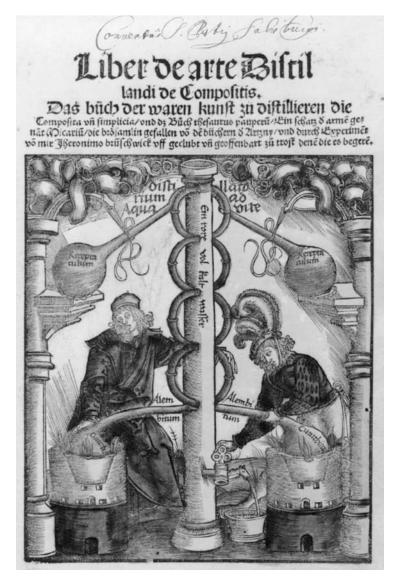
**FIGURE 99.** ■ Title page (hand-colored; see color plates) from *Liber de Arte Distillandi* (Heironymous Brunschwig, 1512), depicting a double-still in which the central tower contains cooling water that is continuously replenished. Come to think of it, this apparatus evokes an image of the caduceus: two serpents entwined about the staff of Hermes where the loops symbolize "couplings." (From the Othmer Library, CHF.)
