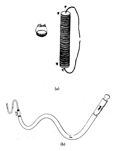
**FIGURE 245.** ■ From Humphry Davy, *Elements of Chemical Philosophy* (Philadelphia & New York, 1812; first English, London, 1812): (a) Davy's voltaic pile consisting of alternating zinc and silver plates separated by moistened cloth; (b) another gun-barrel experiment. In the white-hot gun barrel (free of air), potash yields metallic potassium; potassium was first generated using the voltaic pile. When he discovered potassium Davy "... actually bounded about the room in ecstatic joy."
