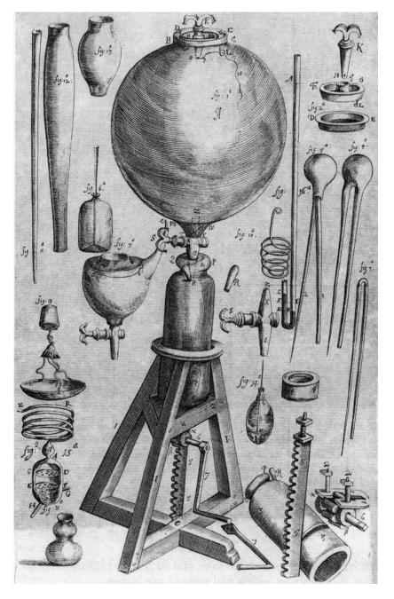
**FIGURE 145.** ■ The Boylean vacuum pump, built by Robert Boyle's assistant Robert Hooke (from *New Experiments Physico-Mechanical, Touching The Spring of the Air,* 2nd ed., London, 1662).
