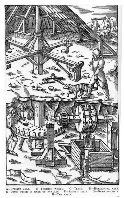
**FIGURE 20.** ■ A horse-driven apparatus for pumping water out of mines (from the 1912 Hoover translation of Agricola's 1556 *De Re Metallica*). Agricola believed in mine goblins whose emanations (carbon monoxide?) were deadly to miners.
