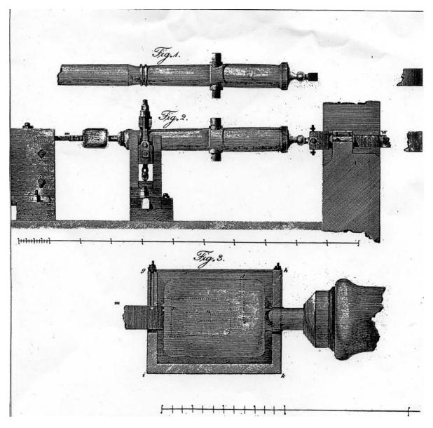
**FIGURE 222.** ■ The cannon-boring experiment of Benjamin Thompson (Count Rumford), which disproved the caloric theory (from *Philosophical Transactions of the Royal Society of London*, Vol. 88 (1798) pp. 80–102).
