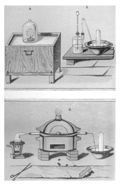
**FIGURE 251.** ■ Black and white image of a color plate from the 1854 American edition of *Notions Générale de Chimie* by Pelouze and Fremy. See color plates. Depicted in 4 is the combustion of phosphorus in air leaving unreactednitrogen; 5 shows the generation of hydrogen through reaction of zinc and sufuric acid—work first published by Henry Cavendish in 1766. In 6, we see Lavoisier's decomposition of water using an iron wire in a porcelain tube heated red hot in a furnace (see Figure 204).
