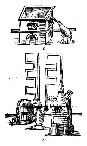
**FIGURE 114.** From French's *The Art of Distillation:* (a) Apparatus for distilling spirit of salt (hydrochloric acid), a very biting "serpent" indeed; (b) State-of-the-art still with water-cooled condenser for distilling volatile liquids. Similar apparatus are still found in the hills of Kentucky and West Virginia.
